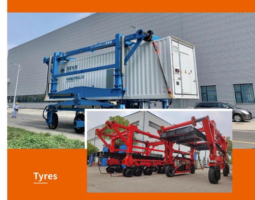
According to your requirement, SPEO can offer designs on different tyre format with 4/6/8 or more tyres for the Straddle Carrie to fit your ground conditions.
