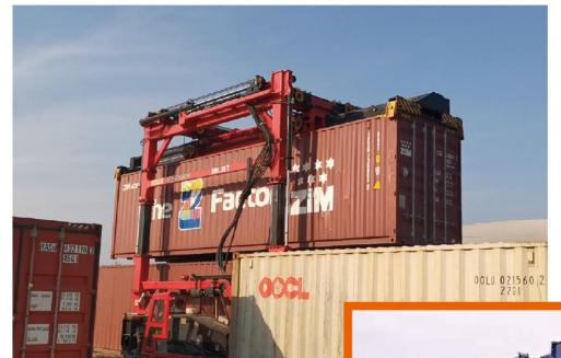
Campared to 80T Reach Stacker, SPEO Straddle Carrier main machine only weighs 18T.The light weight provides much adavatages in cost and daily consumption.
